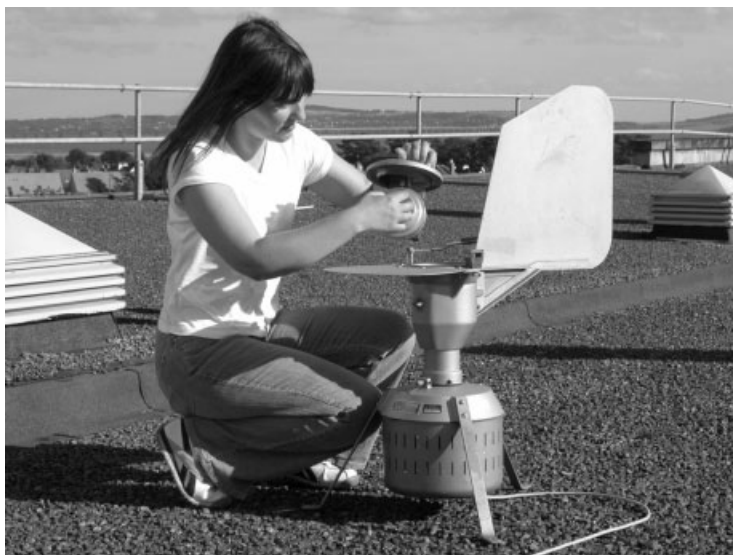
Figure 3.2 A Burkard volumetric spore trap in use for pollen monitoring.
